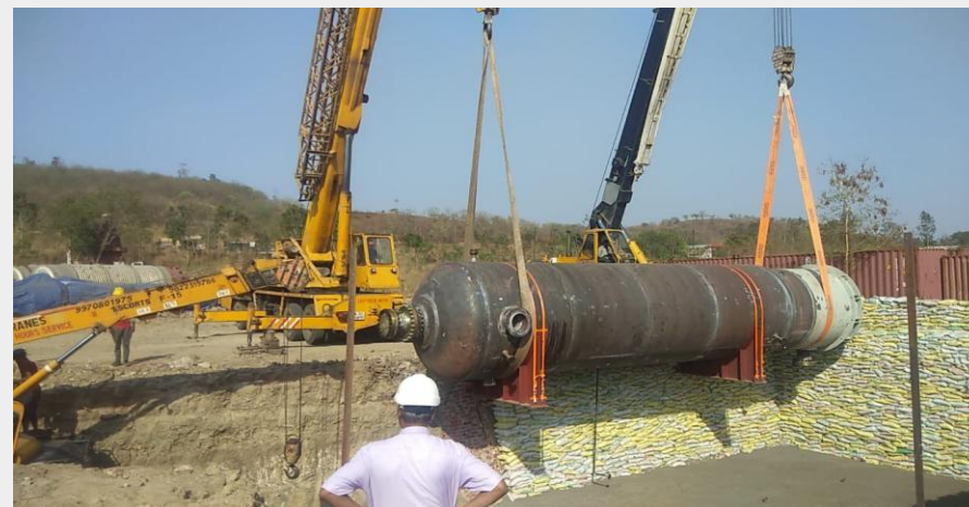
Pneumatic pressure test @40 Bar
