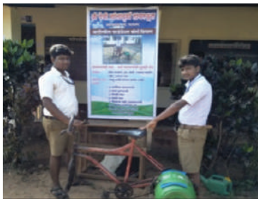
Manually operated low cost washing machine prepared by IBT students
